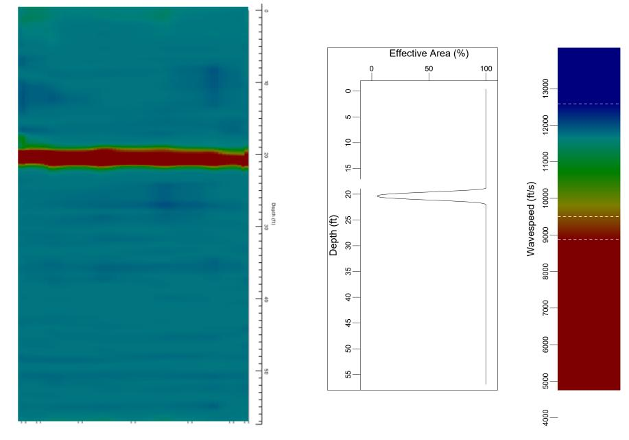
Effective Area is the percentage of cross-sectional area with wave speeds greater than the effective wave speed (EWS) selected by the user, 9500 ft/s
